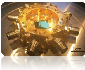
Measurement box containing a chip with superconducting resonators
