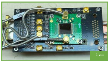
Wired sample before cryogenic cooling
